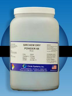
Sir-Chem<sup>®</sup> Dry Powder 68 is a highly refined nonfluorescent blue magnetic powder used for dry method magnetic particle inspection. It is designed to be used in visible light to reveal minute discontinuities on fabricated components or weldments such as bridges, pipes, large tanks, machinery and equipment.
